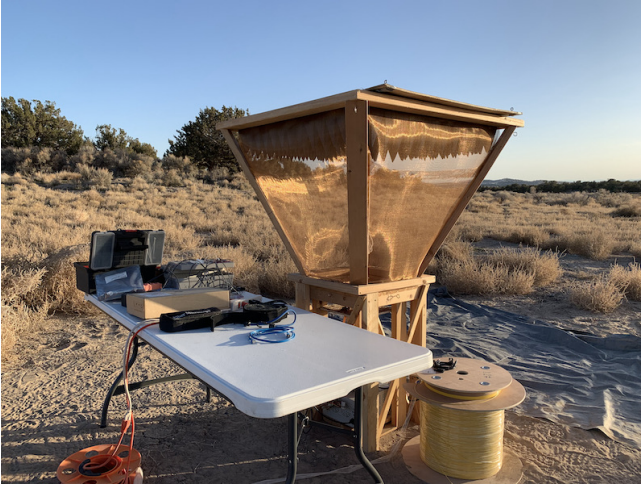
Figure 4. Equipment at the remote measurement site with the conductive ground shield setup for a hot load antenna measurement for the Y factor method.
