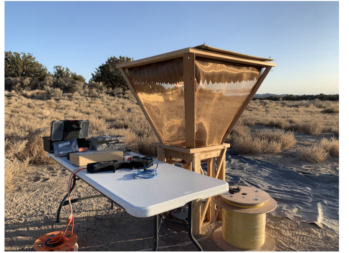
Fig. 1. Equipment at the remote measurement site with the conductive ground shield setup for a hot load antenna measurement for the Y-factor method.
