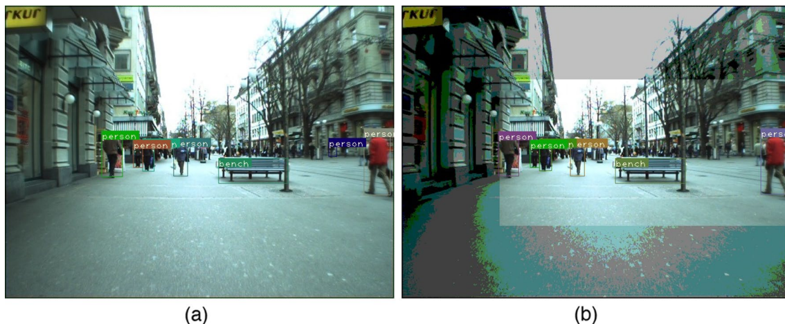
Fig. 10 a Object detected on original image with uniform bit-width (MOT17). b Object detected for image ROI extracted images (bit-width ratio of non-ROI/ROI = 0.25)
