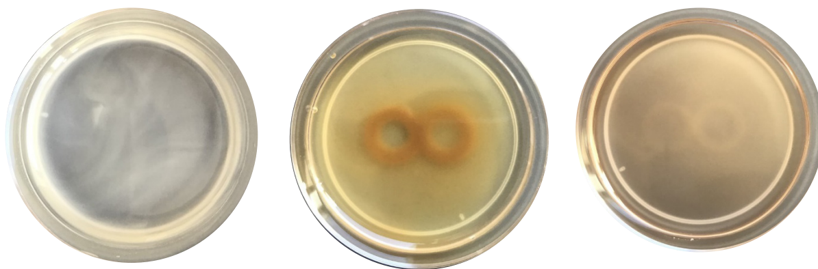
Figure 5. Yeast migration towards two ring shaped magnets with control plate, \text{FeCl}_3 treated yeast and \text{Fe}(\text{maltol})_3 treated yeast.
