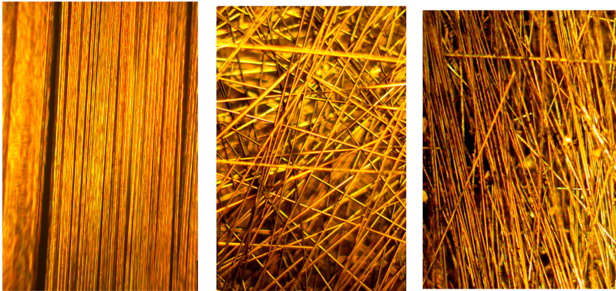
Fig. 6. Aligned virgin fiber (left), non-aligned recycled fiber (middle) and aligned recycled fiber (right). (For interpretation of the references to colour in this figure legend, the reader is referred to the web version of this article.)
