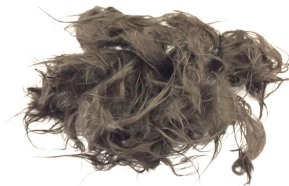
Fig. 1. As-received recycled carbon fibers resemble cotton candy of highly entangled fibers.
