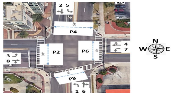
Figure 4. Four pedestrian phases, P2, P4, P6, and P8, and the eight vehicle phases, 1, 2, 3, 4, 5, 6, 7, and 8, are shown for University Ave & 13 th St.
