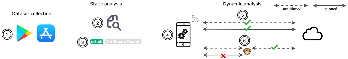
Figure 1: Our methodology to detect certificate pinning. We (1) crawl Android and iOS apps, (2) search app contents for certificate files or hashes, (3) retrieve certificates corresponding to the hashes using publicly available Certificate Transparency logs, (4) launch every app on a real device and collect network traffic in two distinct settings: (5) when app traffic is not intercepted, and (6) when app traffic is intercepted through monkey-in-the-middle (MITM) technique. We identify and mark TLS connections that transmit data in the former setting but not the latter as pinned.
