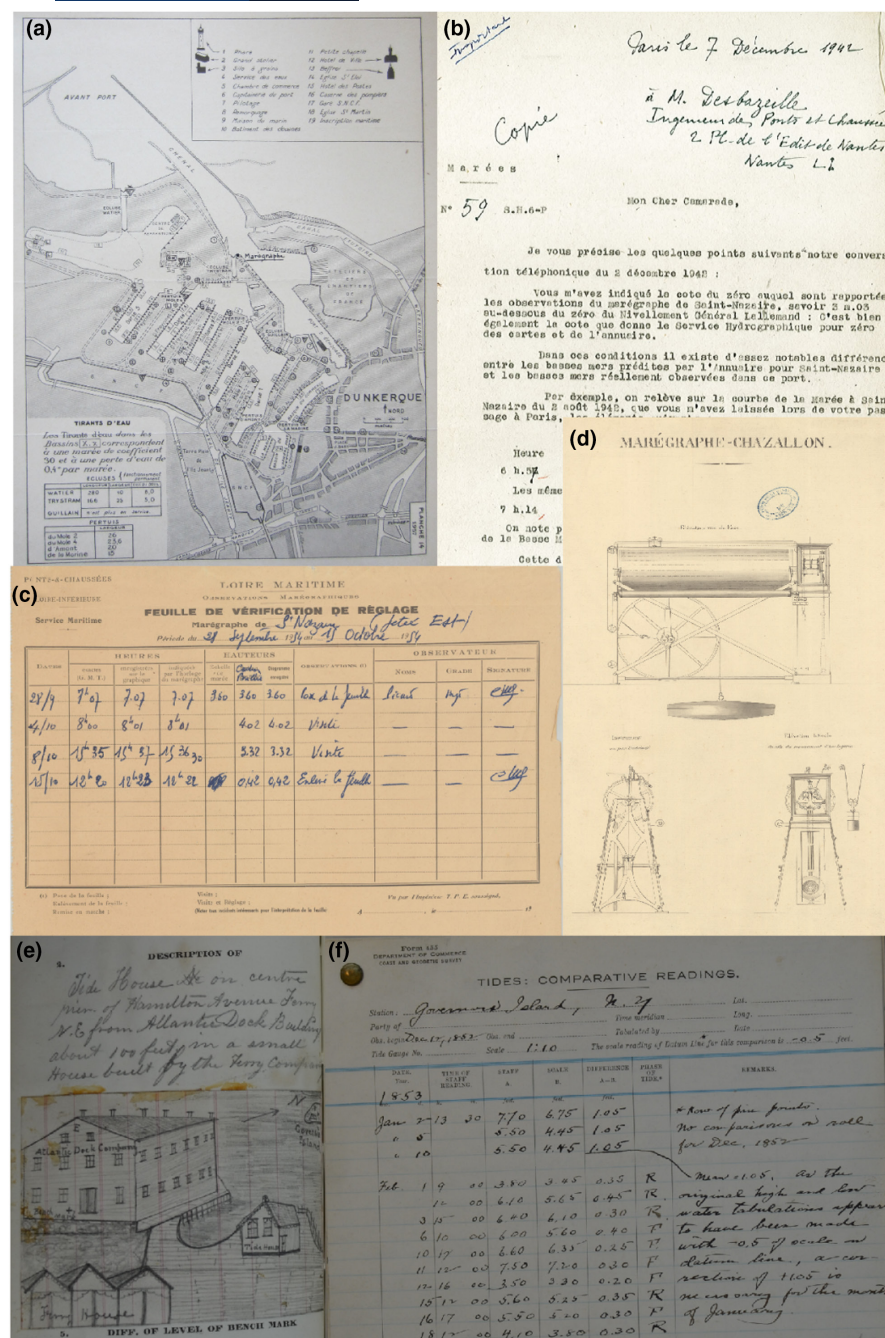
FIGURE 3 Different type of ancillary documents: (a) plan of the location of the tide gauge in Dunkirk (source IGN, boîte 1,346); (b) letter reporting the levelling between the St-Nazaire tide gauge datum and the geodetic network of the time in 1942 ('Nivellement Général Lallemand'; source: Shom); (c) control sheets of the Saint-Nazaire tide gauge in 1954 (source: Grand port maritime de Nantes Saint-Nazaire); (d) 'Chazallon tide gauge' plan (source: Shom); (e) Drawing of the location of the new tide house of Brooklyn made the 27th August 1861 (source: Record group 23 [hydrographic records of the US coast and geodetic survey] in the US National Archive at College Park, Maryland. Photo credit: Patrick Lau); (f) Comparison between automatic tide gauge heights and those read on the scale at the Governor Island station in 1853 (source: Record group 23 [US coast and geodetic survey], in the US National Archive at College Park, Maryland. Photo credit: Stefan Talke/Patrick Lau)
