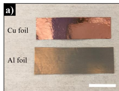
FIGURE 1: Image of commercially procured and annealed a) Copper (Cu) foil, and b) Aluminum (Al) foil. Scale bar is 2 cm.
