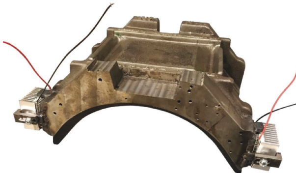
Figure 1. TEG and heat sinks mounted on the bearing adapter. The associated harvesting electronics and instrumentation were mounted offboard to allow real-time performance monitoring.
