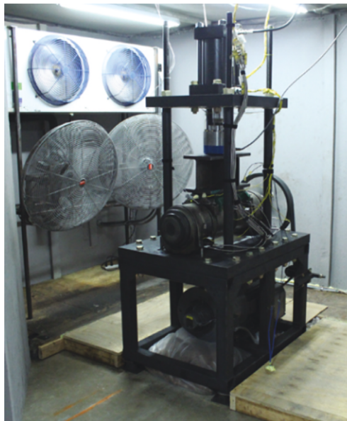
Figure 5. Four bearing dynamic test rig housed in an environmental chamber capable of producing ambient temperatures as low as -40^{\circ}\text{C} and as high as 60^{\circ}\text{C} .
