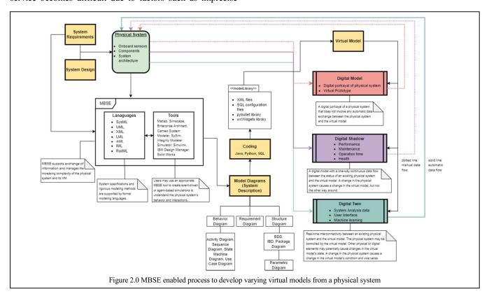
Second, modeling tools can then be implemented to conform with the standards of a specified modeling language, allowing users to build complex model diagrams. Every time a user makes a change to a feature on a diagram created by a modeling tool, it is then changed to the specific diagram itself and other connected model diagrams. This interconnectivity allows for an organized and streamlined system design and implementation process.
