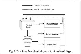
elements, such as the environment of a physical system, may affect the status of the DT as information is automatically transmitted through a database. A change in the physical system causes a change in the DT state and vice versa as represented by Figure 1.
