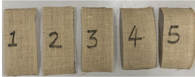
Figure 5. Woven jute fibers cut for tensile tests.
