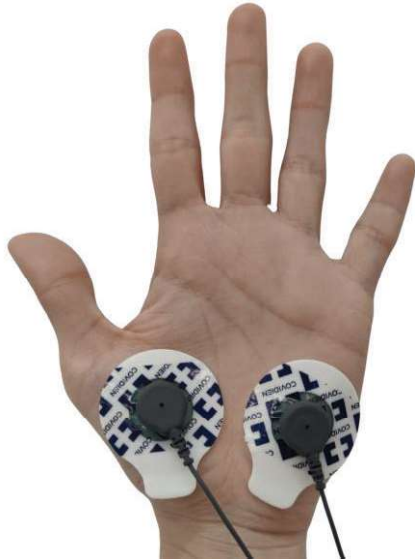
Figure 3. GSR sensor placement diagram
