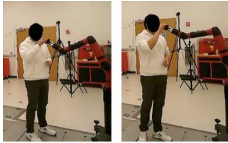
Figure 7. Left: The optimized posture in original RULA. Right: The optimized posture with doubled weight on neck angle.
