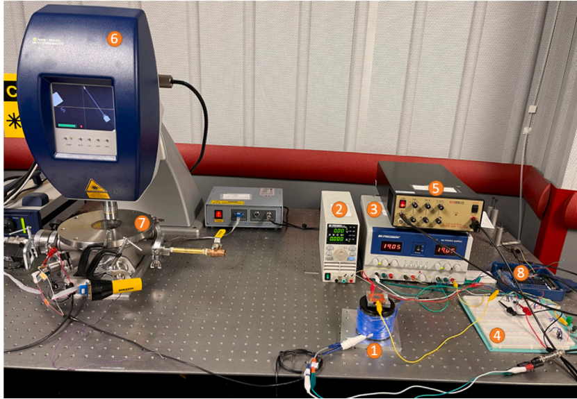
Fig. 3. Testing setup including: (1) Micro triboelectric generator mounted on electrodynamic mini-shaker. (2) DC power supply for generating V_{DC} . (3) Dual DC generator for supplying the summer circuit. (4) Inverting summer circuit. (5) Voltage amplifier for supplying the shaker. (6) Laser vibrometer. (7) Capacitive MEMS switch in the chamber. (8) Data acquisition system.
