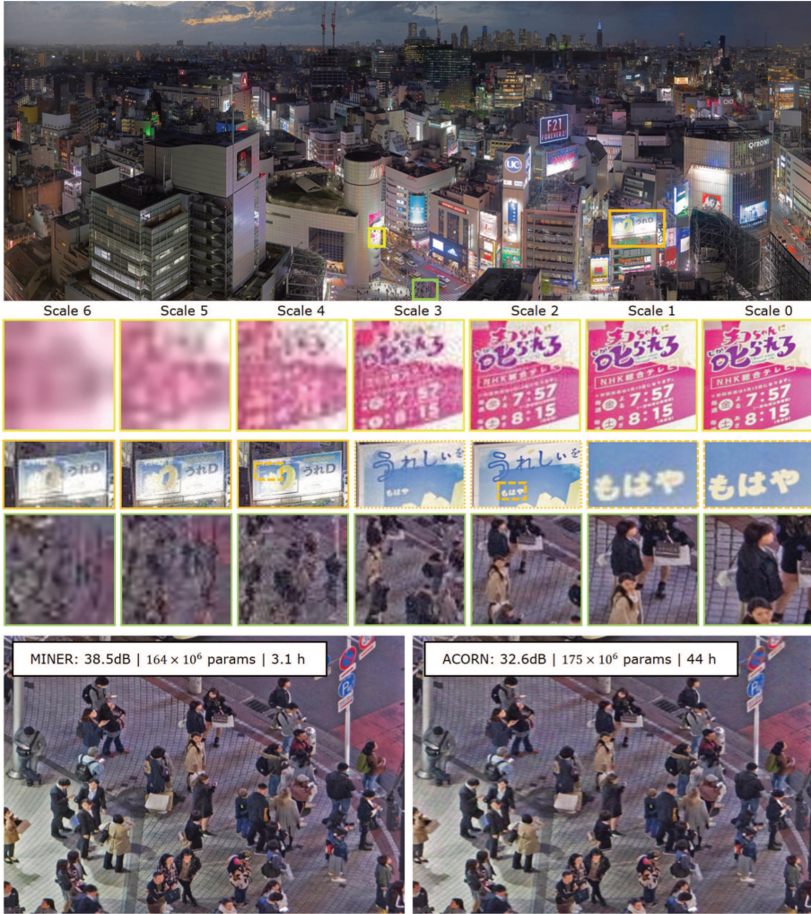
Fig. 7. Fitting gigapixel images. The figure shows the results on fitting a gigapixel image ( 20,480 \times 56,420 ) with MINER and ACORN. MINER required 188 million parameters and converged to 38.5 dB in 3.1 h. In contrast, even after 44 h of training, ACORN, which required 175 million parameters, achieved only 32.6 dB.
