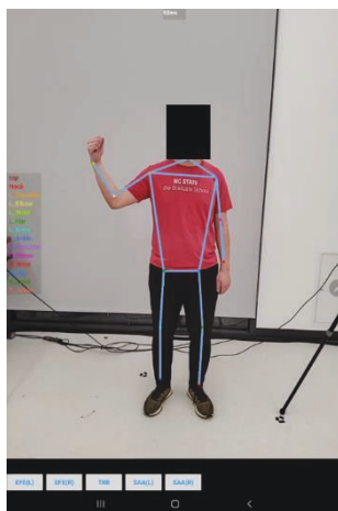
Figure 5. A screenshot of the user interface. The legends of 14 key points are displayed at the center-left. The bottom buttons are EF/E L (left forearm flexion/extension), EF/E R (right forearm flexion/extension), TLB (trunk lateral bending), SA/A L (left upper arm flexion/extension), and SA/A R (right upper arm flexion/extension), respectively.
