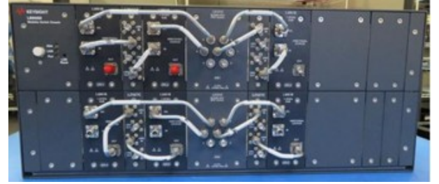
Figure 7: RF Switching Matrix
