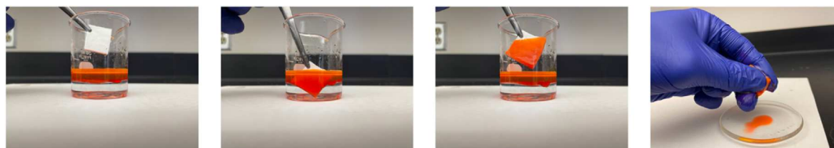
Fig. 4. Representative images of the oil absorption behavior of a pristine PDMS polyHIPE. The white paraffin oil was dyed with Nile red for clarity. Left to right: PolyHIPE before being immersed in the oil/water mixture; polyHIPE wicks up the oil; polyHIPE after being partially filled with oil; polyHIPE being squeezed and releasing the oil. (For interpretation of the references to color in this figure legend, the reader is referred to the Web version of this article.)
