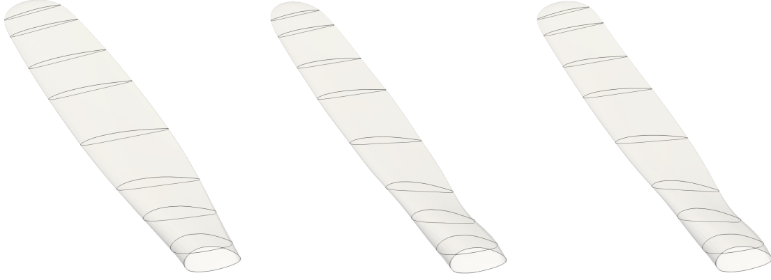
Fig. 14 Comparison of airfoil profiles on the baseline (left), Propeller-only optimization (mid), and propeller-wing coupled optimization (right) designs at different spanwise sections.
