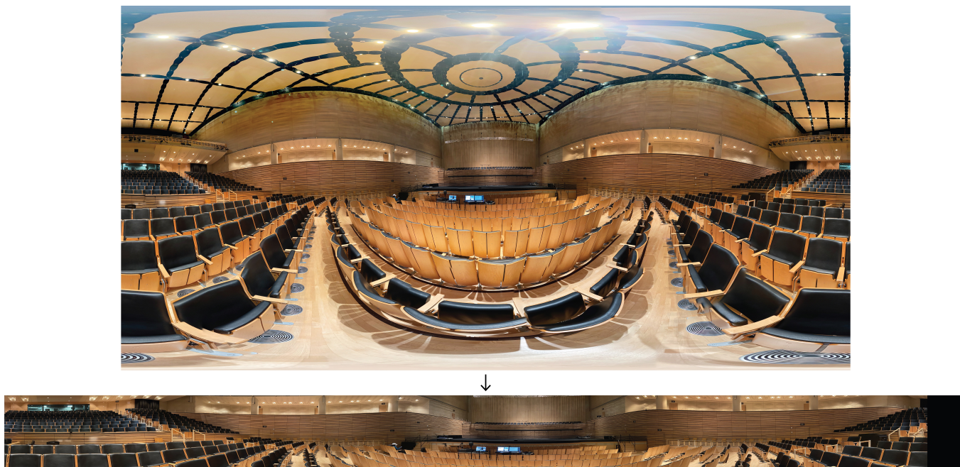
FIG. 8. A standard equirectangular image, above, before it is processed at the back-end through the required perspectival transform and horizontal stretch, below. This correction counteracts any introduced distortion due to the screen's irregular geometry (i.e. rectangular with round corners rather than cylindrical).
