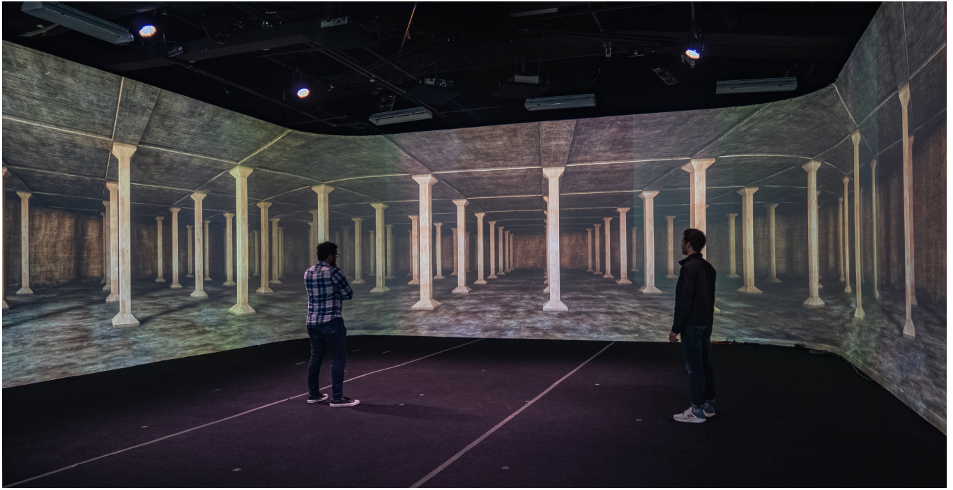
FIG. 1. The Collaborative-Research Augmented Immersive Virtual Environment (CRAIVE-Lab) at Rensselaer is equipped with a nearly-360° front-projection screen. It is microperforated so as to remain acoustically transparent to the dense 128-loudspeaker array located behind it. These systems together present congruent audio-visual content and are utilized for producing walkable auralizations for the purpose of experiential acoustics education.
