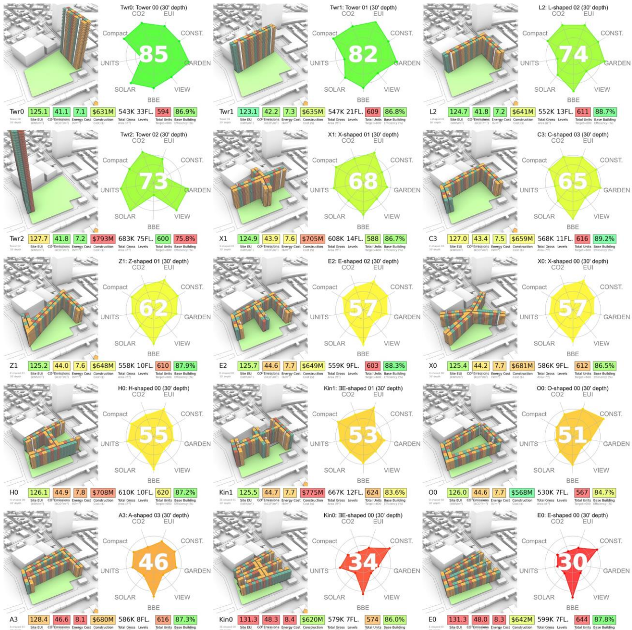
Figure 5: Examples of generated performance evaluation datasets using our program's auto-generated pre-defined built forms. Each example shows a perspective of a building layout (left), a radar chart for nine criteria with an overall score (right), and values from the analysis used for the radar chart prior to normalization (bottom). (Notes: The results are based on the test site in the temperate climate zone on the East Coast of the United States, with the conditions set based on 600 units with percentages for unit types of 20% studio, 36% 1-bedroom, and 44% 2-bedroom apartments).
