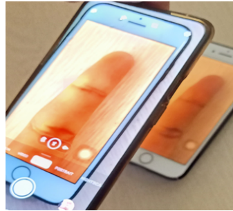
Figure 1. An example of a finger photo display attack. A finger photo of the genuine identity is displayed by using a smartphone positioned in front of the camera integrated in the mobile to unlock.
