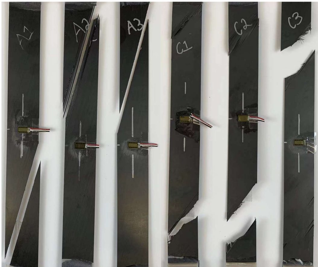
Figure 2. Photograph of specimens after tensile tests, where A1-A3 are auxetic CFRP composite specimens (laminate layup: [15/65/15/65/15] ) and C1-C3 are non-auxetic counterpart CFRP composite specimens (laminate layup: [35/60/-5/60/35] ).
