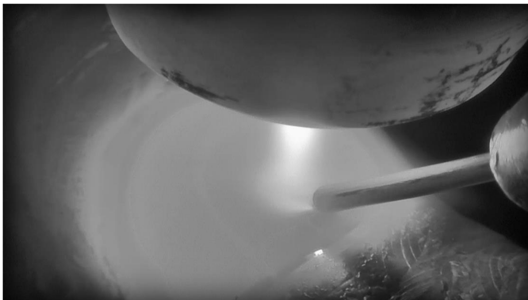
Figure A 5: Video still demonstrating the XY-plane traversal of the deposition process. The central point of the TIG torch never reaches the edge of the build geometry, partially heating both the inner and outer diameters. This results in less heating after initial deposition and the retention of the large colony microstructure. The full video can be seen in Supplementary Materials.
