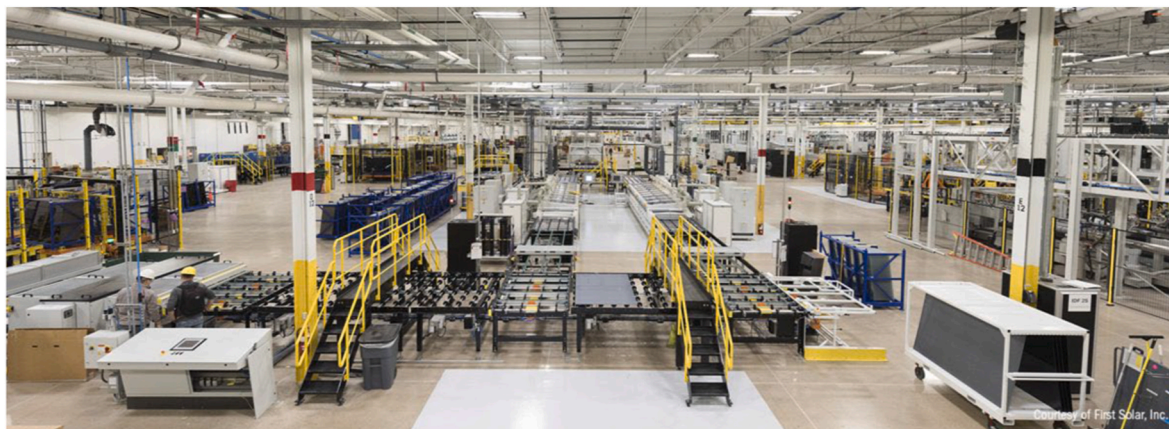
Fig. 7. View of a First Solar manufacturing line. A grey rectangular Series 6 module is visible in the foreground on the conveyance system between the two walkover paths with yellow railings and two workers are present to the left for scale. Hundreds of other nearly-finished modules are visible in the blue metal racks to either side. It is remarkable to note that high-efficiency CdTe modules are produced in factories in which they are transported in open air between process steps rather than e.g. in a cleanroom. Image courtesy of First Solar.
