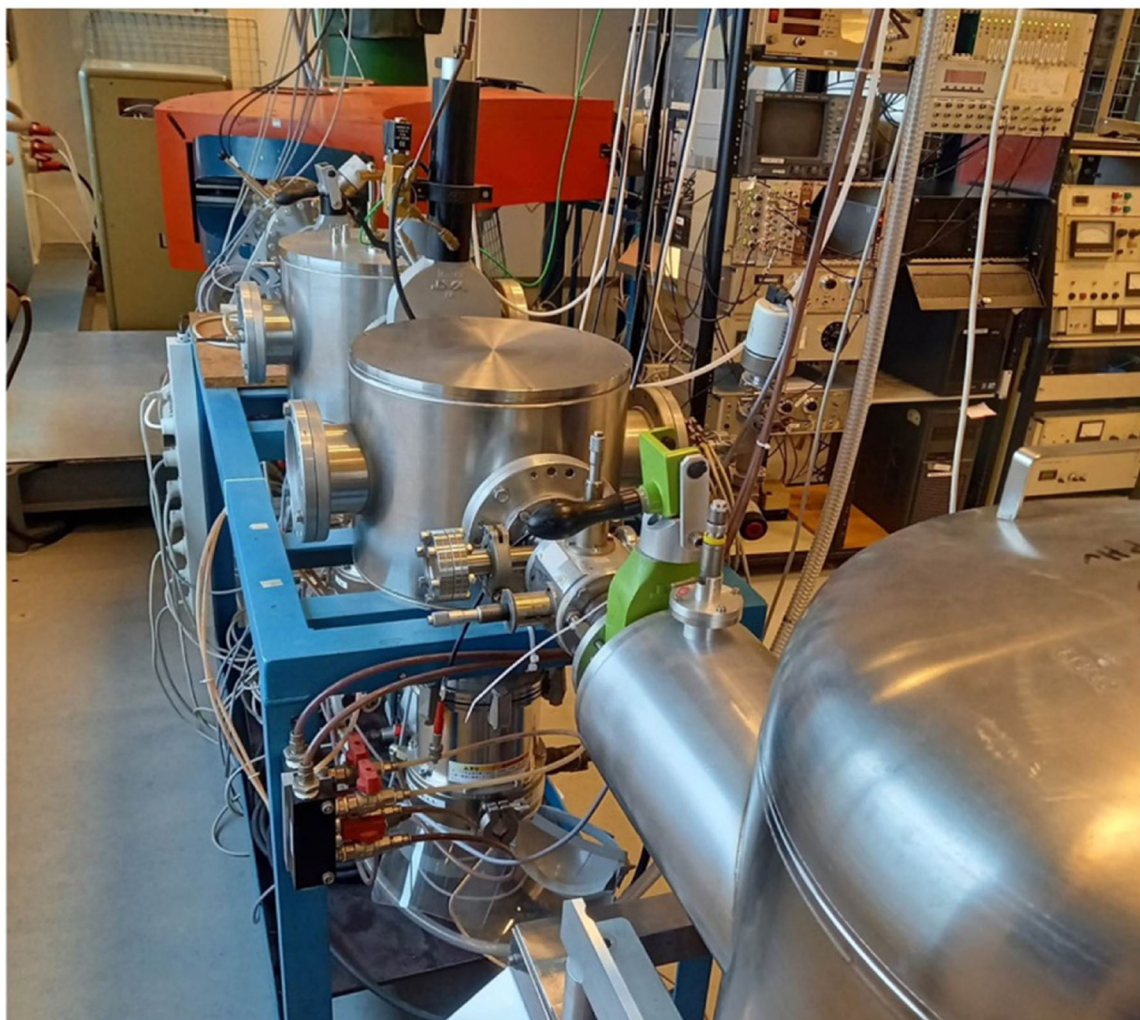
FIGURE 3 Top: Scheme of the Aarhus tandem instrument. Bottom: picture of the photodissociation field-free region containing collision cells [Color figure can be viewed at wileyonlinelibrary.com ]
