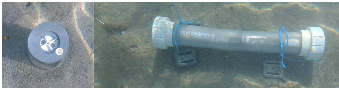
Fig. 8. Benthic flux chamber (left) and PAWS (right) deployed at 1 m water depth in Mo'orea, French Polynesia. The flux chamber consists of a 10 cm clear tube capped with a sealed lid (grey) which contains a manual magnetic stir propeller (center white) and a rubber septum for sampler collection with a syringe (edge white). The chamber is driven into the seafloor to collect potential chemical fluxes over a 12-hour period. The PAWS system was deployed alongside three flux chambers to collect a comparison sample of ambient seawater.
