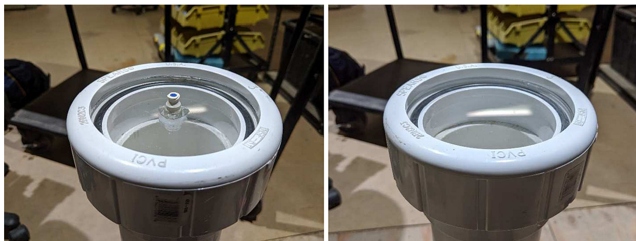
Fig. 6. PAWS housing with PVC union threaded endcaps and collars. The front and rear doors (left and right respectively) are made from laser cut clear acrylic. The pass through in the front door is an IV valve epoxied into a laser cut, or drilled, hole through the center of the disc.
