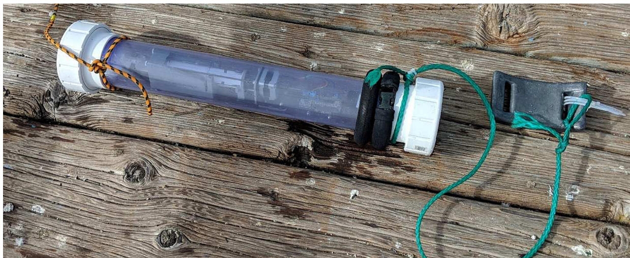
Fig. 1. PAWS on a pier ready for deployment. The black bands are SCUBA diving ankle weights. The dive weight attached to the green rope hits the seafloor before the sampler does allowing PAWS to be anchored above the bottom reducing the possibility of particulate matter blocking the sampler's inlet. (For interpretation of the references to colour in this figure legend, the reader is referred to the web version of this article.)
