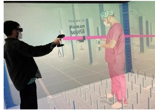
Figure 2. A user in the CAVE. The wand's virtual magenta ray activates interactive 3D user interface elements.
