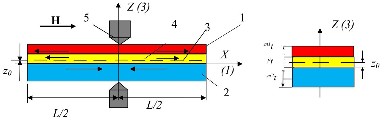
Fig. 1 Schematic drawing of the structure. 1 - magnetic layer 1 (positive), 2 - magnetic layer 2 (negative), 3 - piezoelectric layer, 4 - neutral line, 5 - electrodes.
