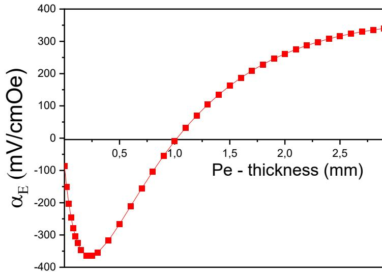
Figure: 2 Dependence of the low-frequency MEVC on the Pe thickness of the for a fixed thickness of the Ni layer  $Ni_t=1.0$  mm and the thickness of the piezoelectric PZT layer  $P_t=0.2$  mm.
