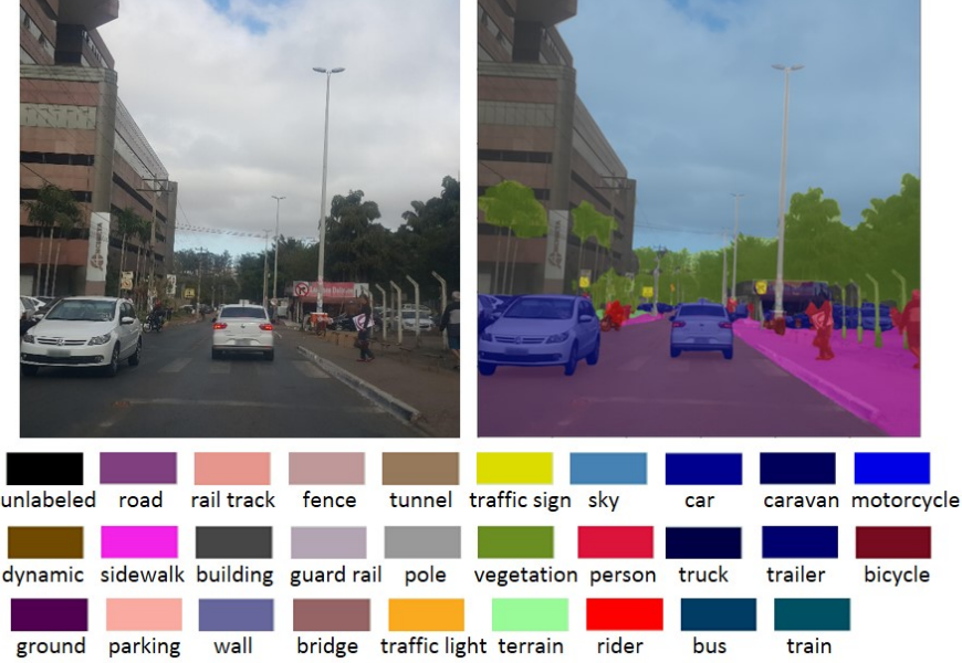
Figure 3: Semantic segmentation results and labels on the Cityscapes dataset using DeepLabv3+. Best view in color.
