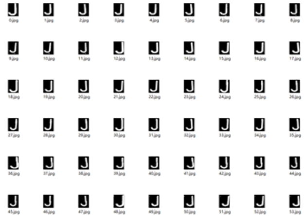
Figure 7: In Order To Improve Accuracy on Character Recognition for License Plates, We Only Use Well-printed Examples for Our Character Recognition Program
