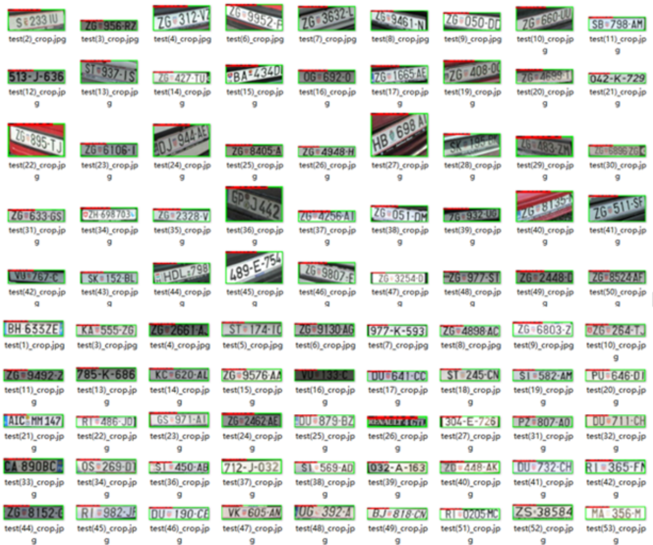
Figure 9: License Plates Can Be Perfectly Detected with Conditions Such As Dark, Bright Environments, Huge Noises, and Some Even Tilted
