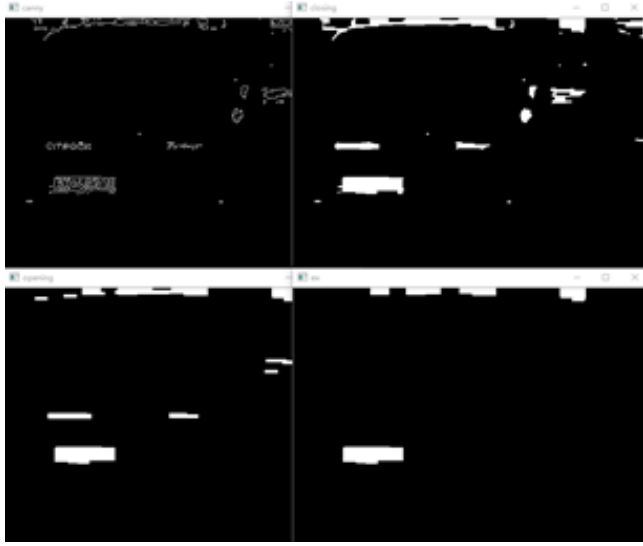
Figure 1: Image Processing Algorithms Extract Plate Features with Gaussian Noise-reducing Filter, Opening, and Closing Operations for Edge Emphasizing
