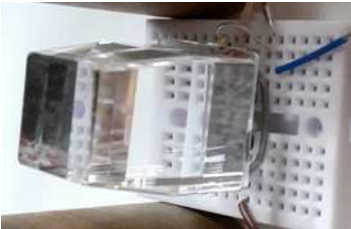
Figure 3. A prototype LYSO crystal readout by a Silicon photomultiplier. The tapered design was selected to cover a larger solid angle, and increase photopeak efficiency compared to a parallelepiped. The crystal is 3 cm along the long axis. This picture does not feature any crystal wrapping.
