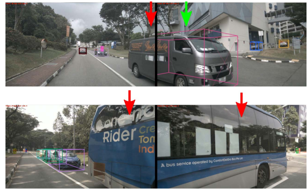
Figure 1. First row: the object detector and tracking method DEFT [5] fails to detect partial objects in one camera but can detect in another camera, Second row: The detector fails to detect objects in both cameras. Green arrow indicates true positive detection sample, red arrows indicate false negative detection samples.
