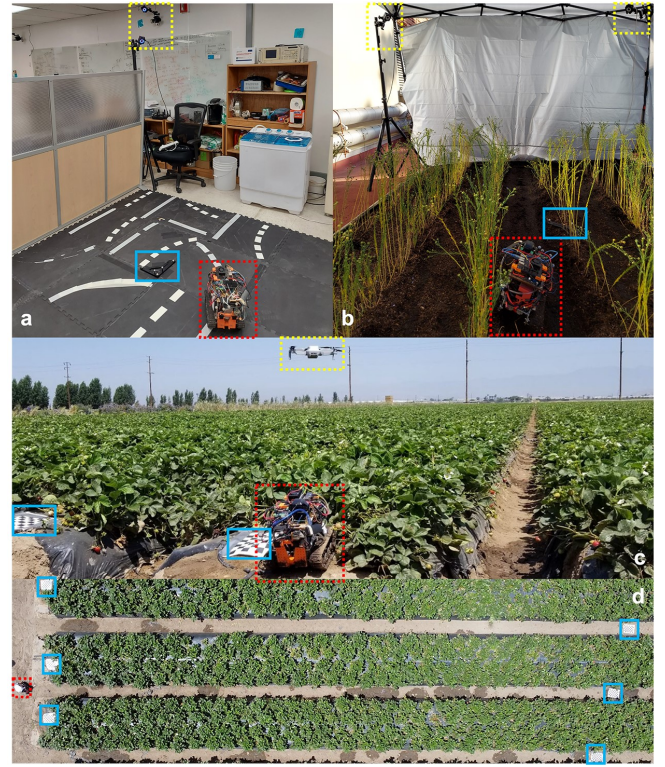
Fig. 1: Data collection setup for the Agrobot dataset. Dotted red insets show the robot, dotted yellow insets show the ground truth setup, and the solid blue insets show the reference landmarks. (a) Phase 1 (b) Phase 2 (c) Phase 3 (d) The robot and the reference landmarks (checkerboard patterns) as viewed from the quadrotor camera in Phase 3.
