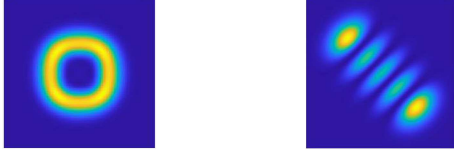
Fig. 3. Simulated mode profile at the focus between the two AMCs (left) and at the VECSEL gain chip (right) under perfect alignment. At the VECSEL gain chip the mode profile was forced to be HG due to the gain modal overlap. This in turn forced the mode profile between the two AMCs to be LG due to the fixed Gouy phase shift relationship between the two planes.
