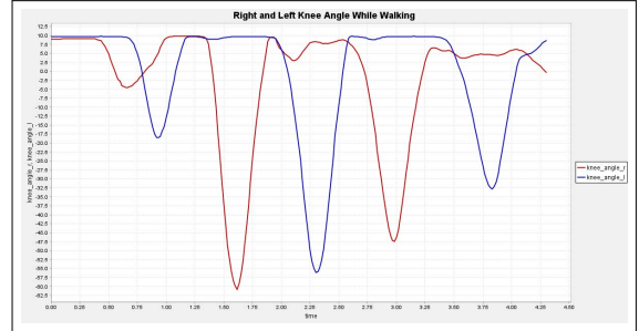
Fig. 8. Rotation angles of the knee joints for the walking volumetric capture
