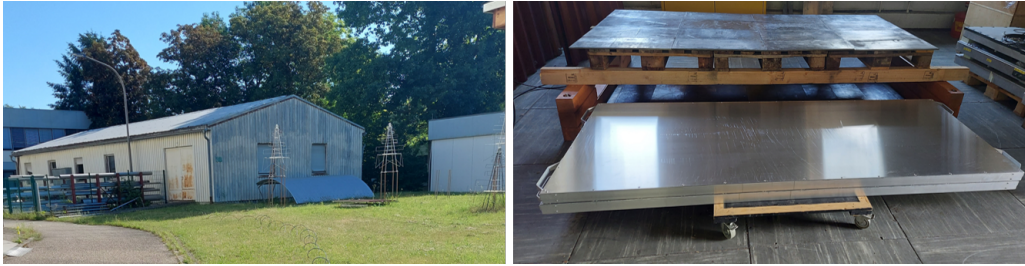
Figure 7: Left: The metal walled building where the test setup is placed. Right: The setup with lead shielding bed on top and bottom. Two panels can be tested simultaneously in this set-up with a slider to position the panels.
