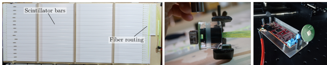
Figure 3: Left: In-lay of the scintillation detectors with the optical fibres. Center: The coupling of the optical fibres to the SiPM. Right: A uDAQ connected to SiPM and the temperature sensor.
