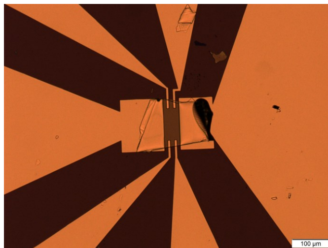
Fig.S1. Optic image of an exfoliated graphite flake with current and voltage leads. Its thickness determined using atomic force microscopy is d = 400 nm. The width and separation between the voltage leads long the current direction are w = 120 μm and l = 18 μm, respectively. The current flows from left to right.
