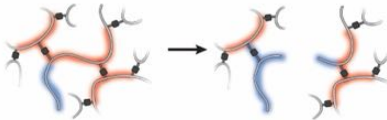
(C) Breaking a strand between two tri-functional crosslinkers
