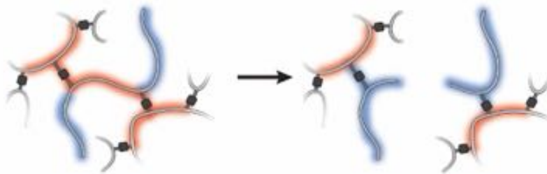
(C) Breaking a strand between two tri-functional crosslinkers
