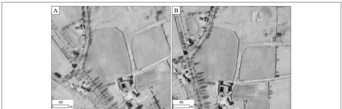
Figure 3. An image quality comparison between 0.50 (A) and 0.61 (B) snapped from 1934 air photos in the same spatial extent. 1934 Aerial Surveys, State Archives Record Group 089:011, State Archives, Connecticut State Library.
