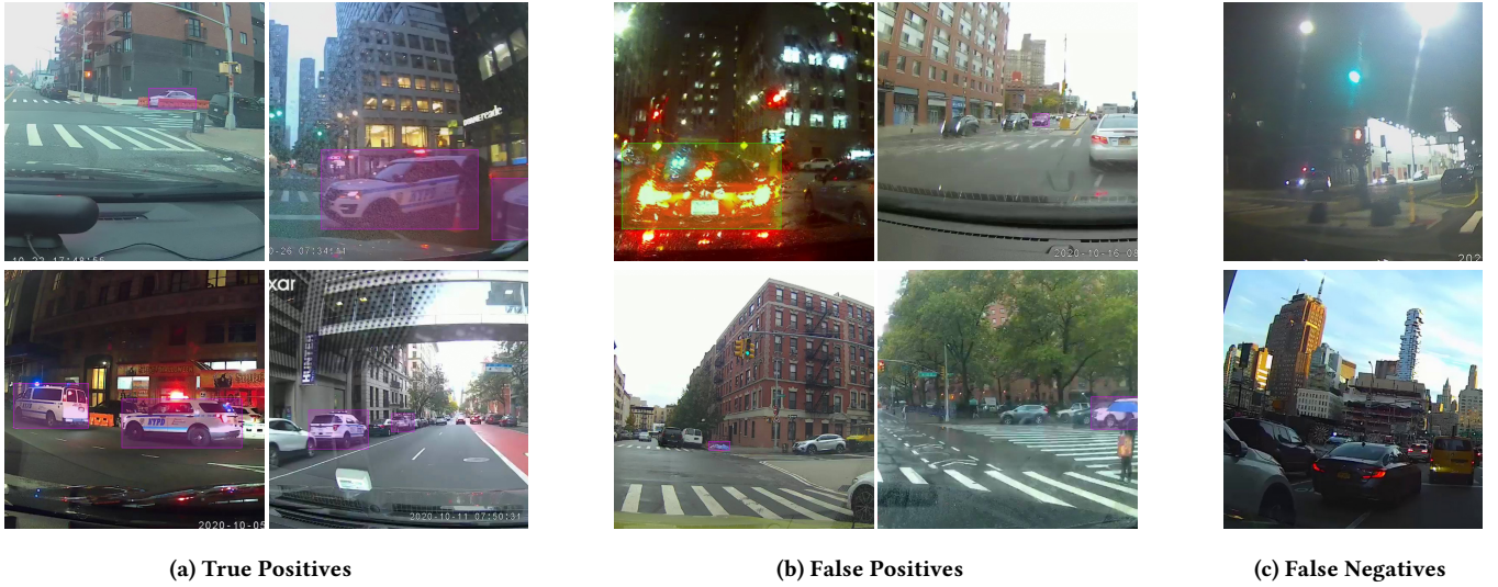
Figure 3: Examples of police vehicle detections. Notice the different times of day, differing camera perspectives, and multiple types of vehicles. Initially, the object detection model was easily confused by NYC taxis, buses, white sedans, and white SUVs. As more training data was added, the model was more difficult to confuse, with incorrect classifications occurring typically with optical illusions and poor light conditions. Note that images are cropped and zoomed to better depict annotated regions; raw images are 1280x720.
