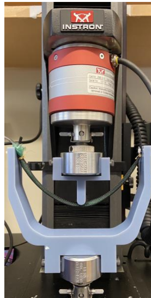
Fig. S5. Modified flex fixture set up. Image of the actuator fixed to a custom 3d-printed modified flex fixture setup used for mechanical characterization and fatigue testing.
