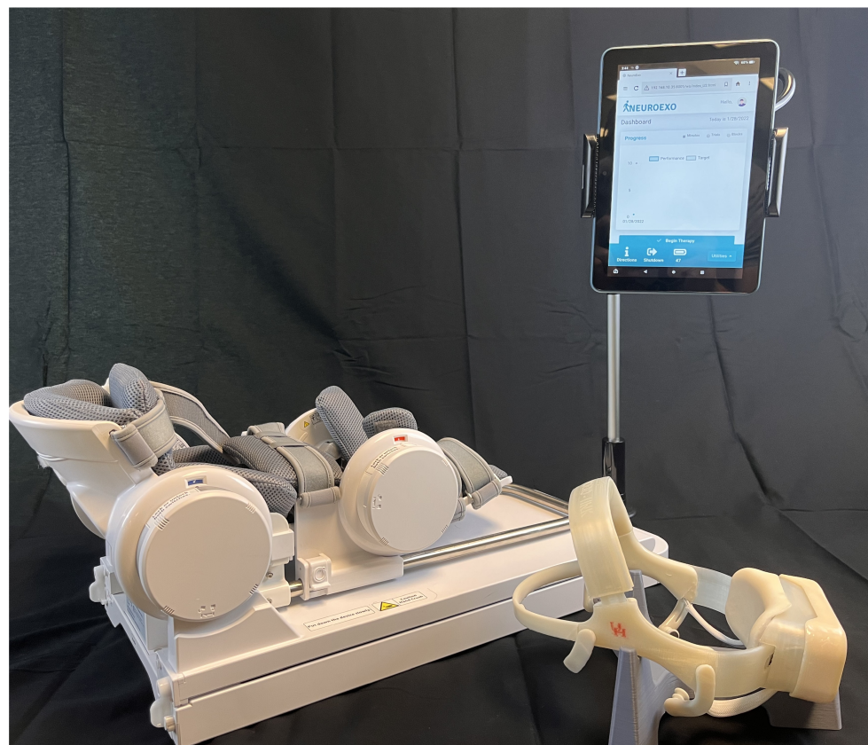
Figure 4. A custom EEG-based BCI headset with wireless tablet-based (Fire 8, Amazon, Seattle, WA, USA) graphical user interface (GUI) and an IoT-enabled powered upper-limb exoskeleton robotic device (Rebless, H Robotics, Austin, TX, USA) deployed in a sample neurorehabilitation application.
