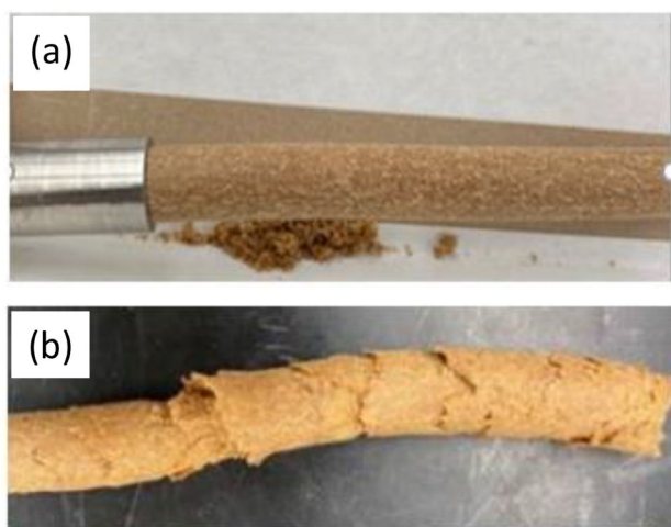
Fig. 7 Photographs of (a) smooth extruded wood-SS (50:50) rods and (b) extruded wood-SS showing sharkskin
