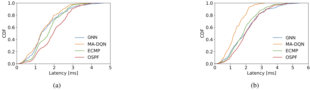
Figure 11: Comparing GCN and MA-DQN: Latency CDF for MA-DQN and GCN models on (a) (50V, 100E), (b) (75V, 150E) Waxman Network.
