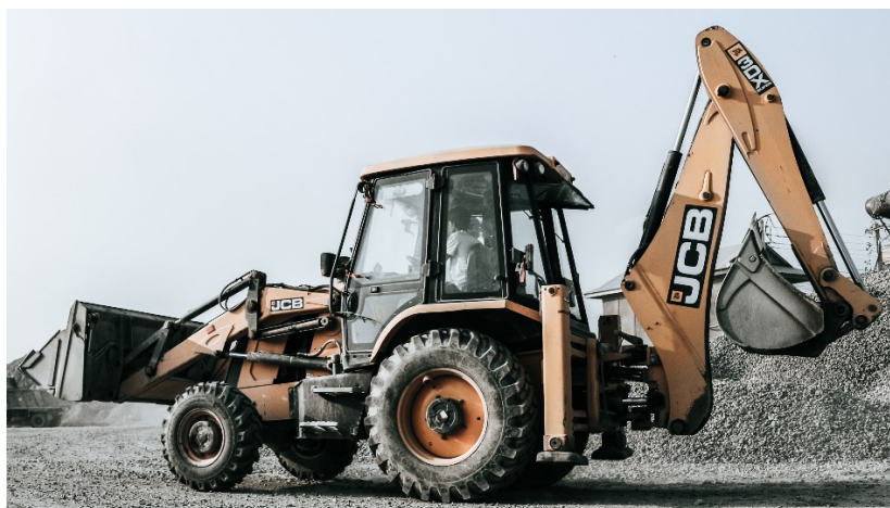
Figure 2. Tractor–loader–backhoes are tractors with a front-mounted loader and a back-mounted backhoe as attachments.
