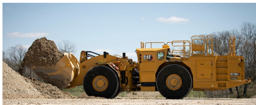
Figure 3. Caterpillar R1700 XE LHD which uses battery-powered electric motors for propulsion [44].
