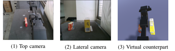
Fig. 5. Initial views of different visualization methods in experiment 1. Method(a), one-image stream(1), includes only the image top camera. Both objects were nearly occluded by the robot arm. Method(b), two-image stream(1+2), includes images from both the top camera and the lateral camera, providing the user with a more comprehensive view of the work space. Method(c), virtual counterparts(only 3), generates the whole object model in VR.
