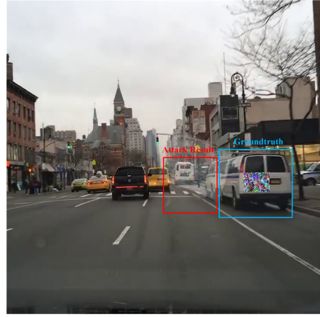
Fig. 4. Move-in attack result using dynamic adversarial patch
