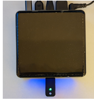
Fig. 4. Solokey hardware security token in use.
